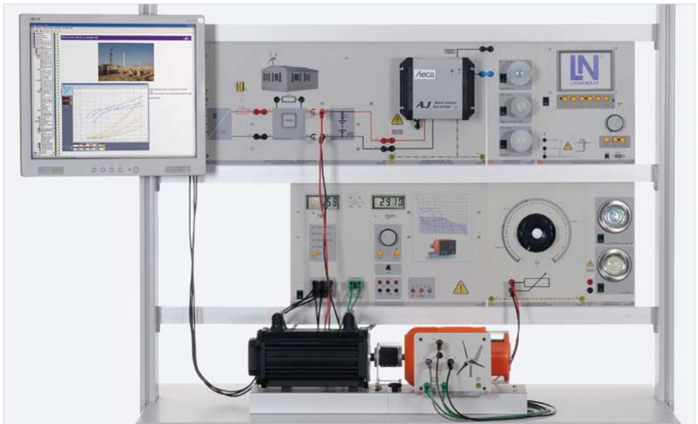
Sample experiment "Small wind power plant" EWG 2
