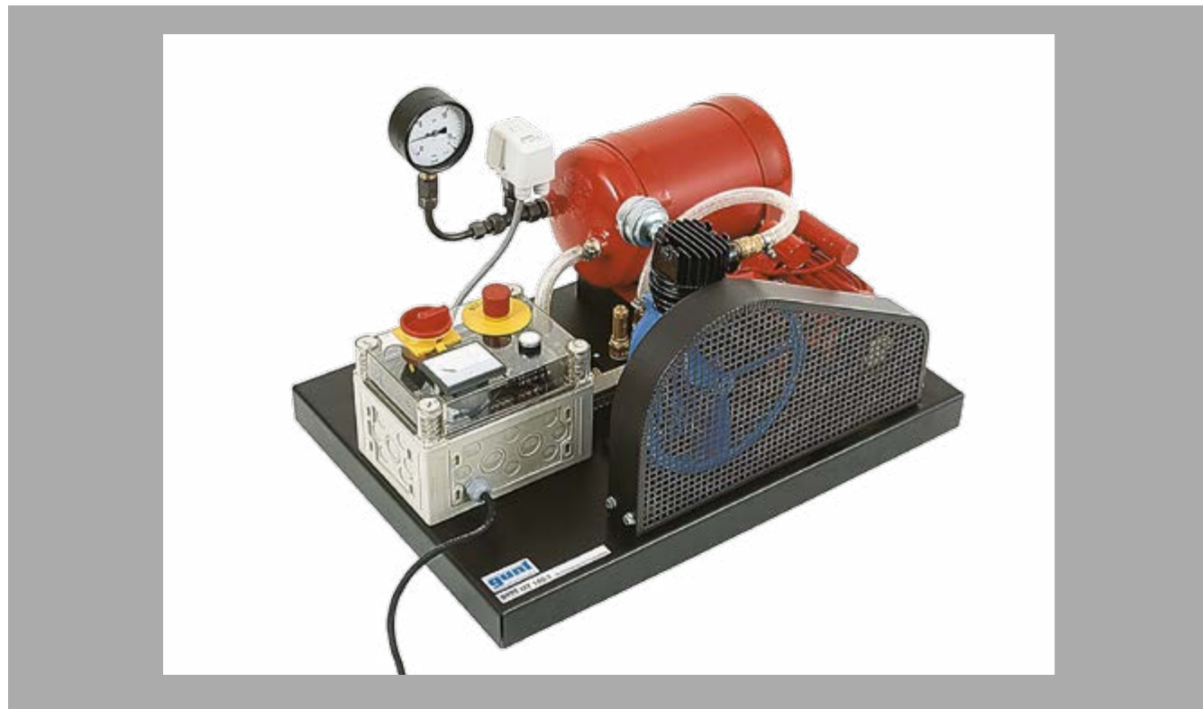
The illustration shows MT 140.01 together with the compressor MT 140.02 under test.
