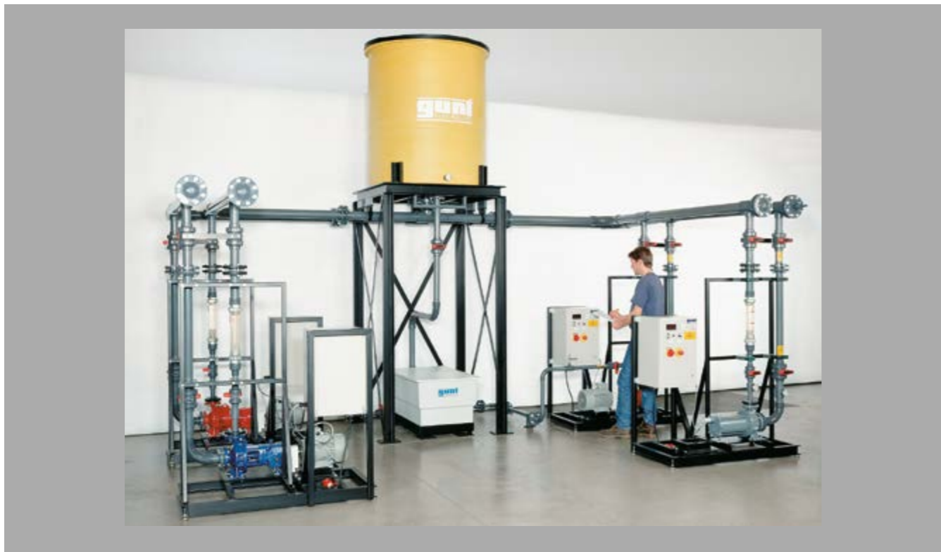
The illustration shows the complete layout of a pump system, comprising four HL 962 assembly stands, each with one pump (HL 962.01 - HL 962.04), the piping system HL 962.32 and the tank system HL 962.30.
