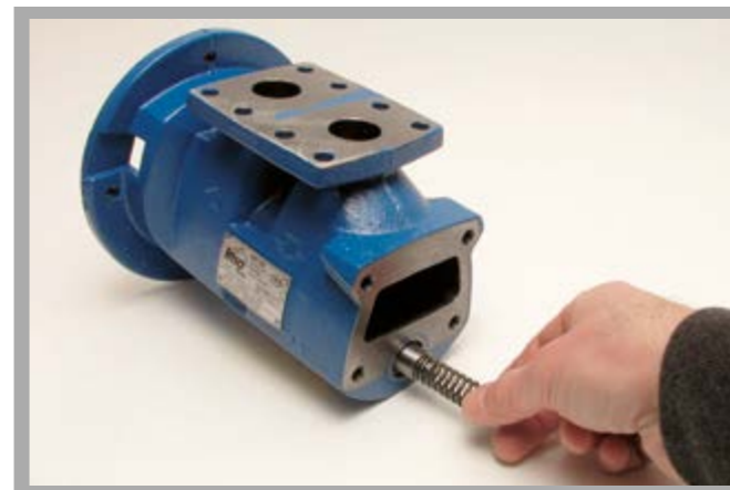
Assembly of the screw pump: assembling the valve piston with the valve spring
