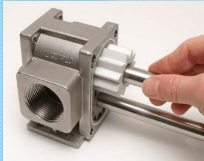
Installing the driven shaft
