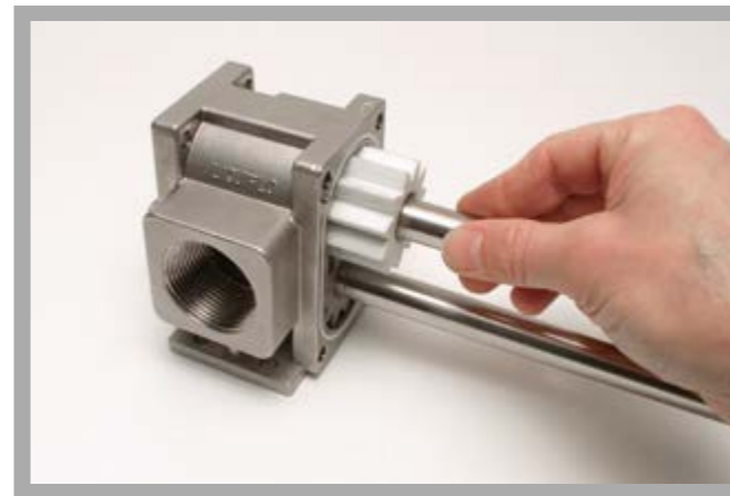
Assembly of the centrifugal pump: assembling the driving shaft
