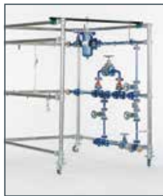
HL 960 Assembly station: pipes and valves and fittings
