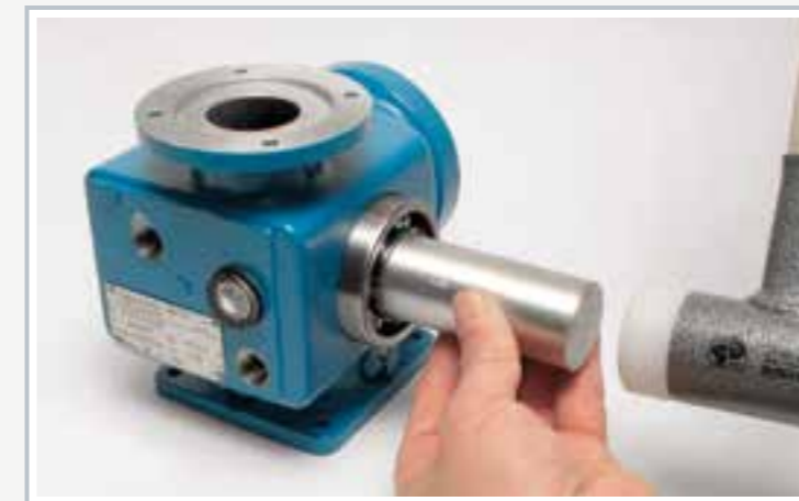
Assembly of the diaphragm pump: driving the eccentric into the housing (using a device)
