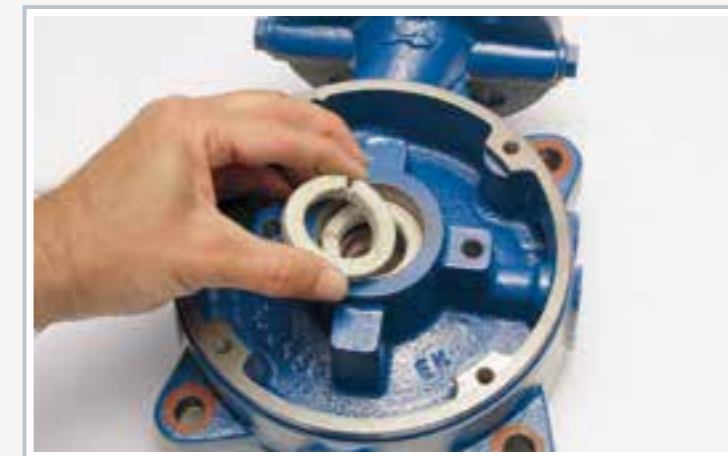
Assembly of the four-stage centrifugal pump: assembling the packing gland rings
