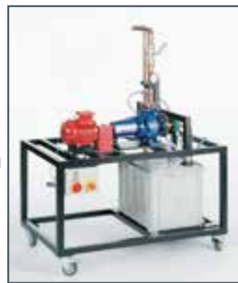
HL 960.01 as closed water circuit
