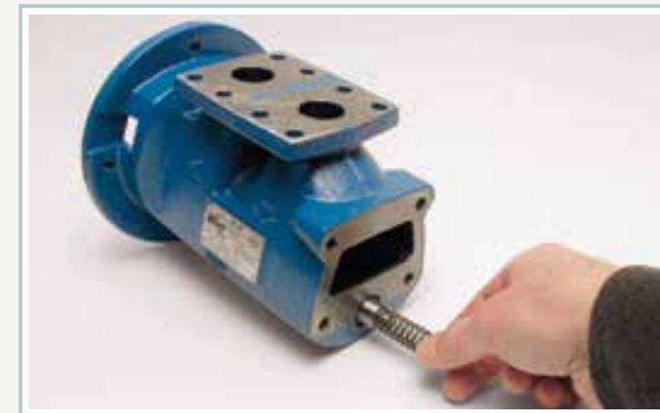
Assembly of the screw pump: assembling the valve piston with the valve spring
