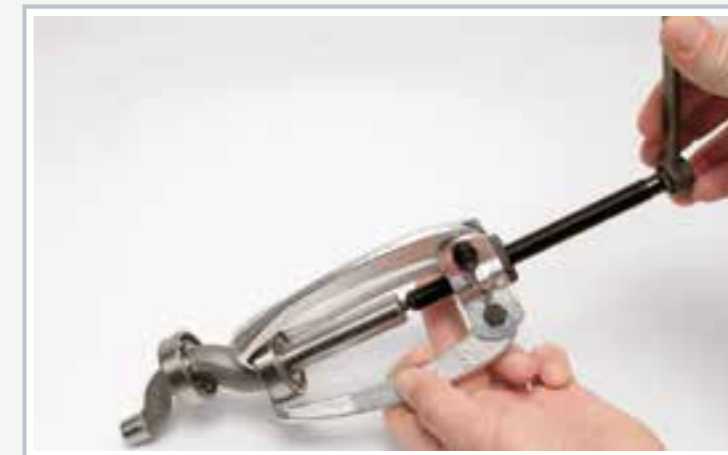
Disassembly of the piston pump: pulling off the ball bearing of the eccentric shaft (using a bearing puller)
