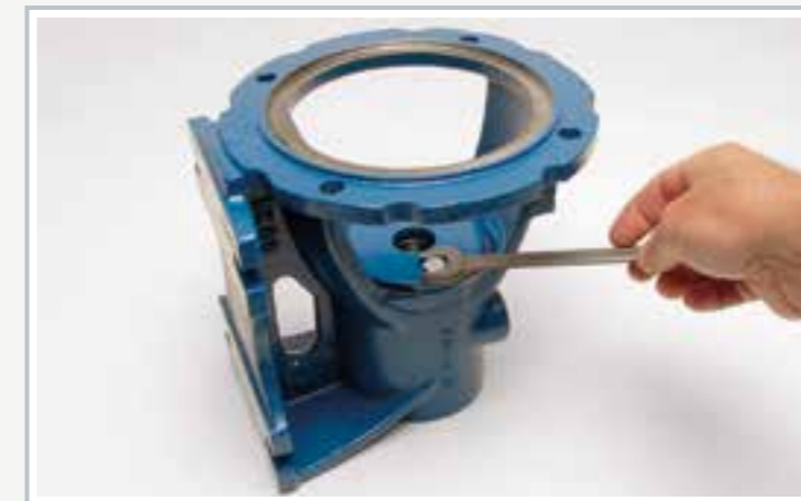
Assembly of the centrifugal pump: fixing of the bearing cover with screws
