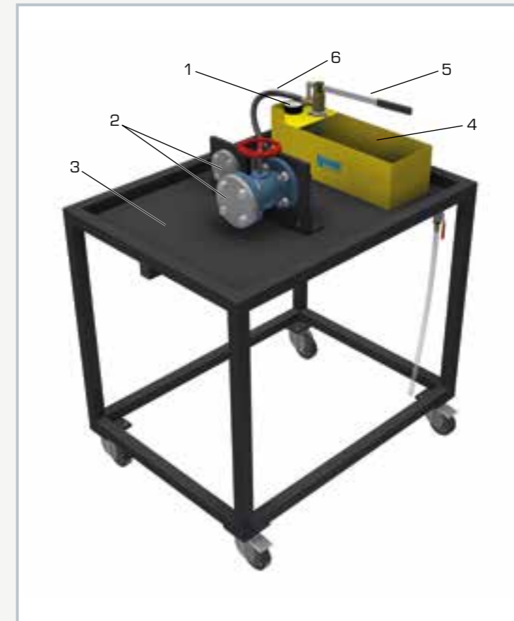
1 manometer, 2 mounting flanges with blank flange, 3 benchtop tray with drain, 4 pressure test pump with water tank, 5 hand lever, 6 hose
