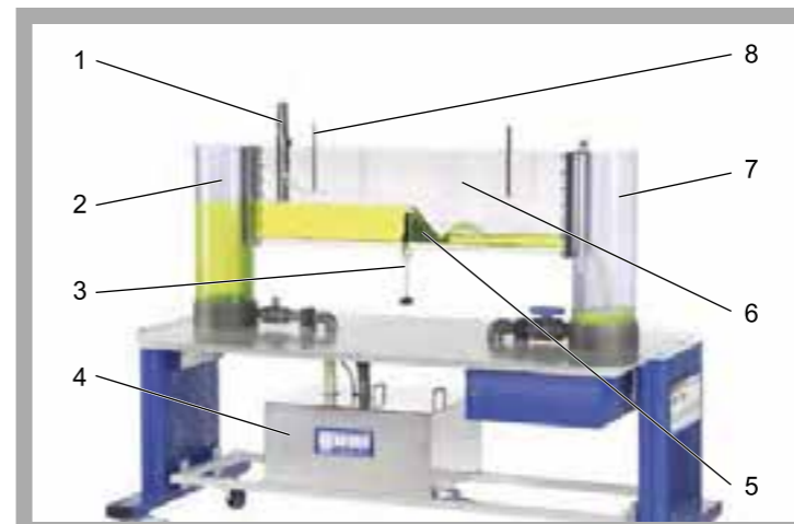
1 sluice gate, 2 water supply, 3 sill height adjustment, 4 supply tank, 5 ogee-crested weir used in the experimental flume, 6 upper limit, 7 water drain with plate weir at the water outlet, 8 measuring tube
