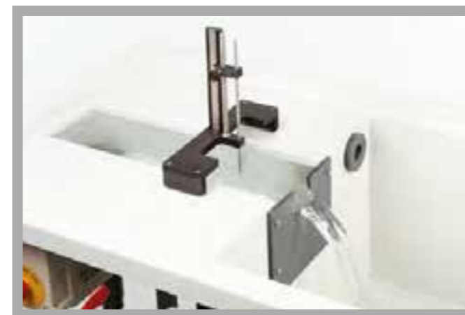
Base module for experiments in fluid mechanics with plate weir HM 150.03
