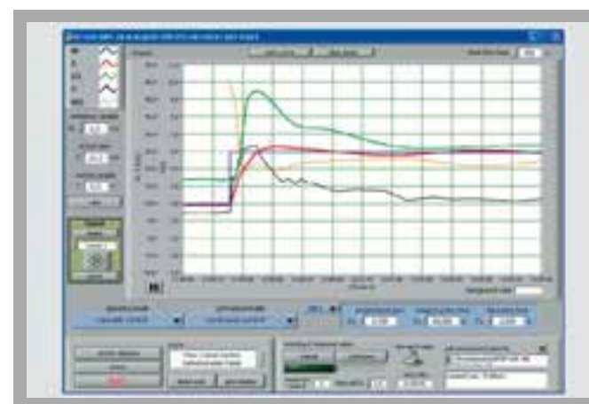
Screenshot of optional I&C software RT 650.40: step response to change in level reference variable with PID controller (acceptable control quality)
