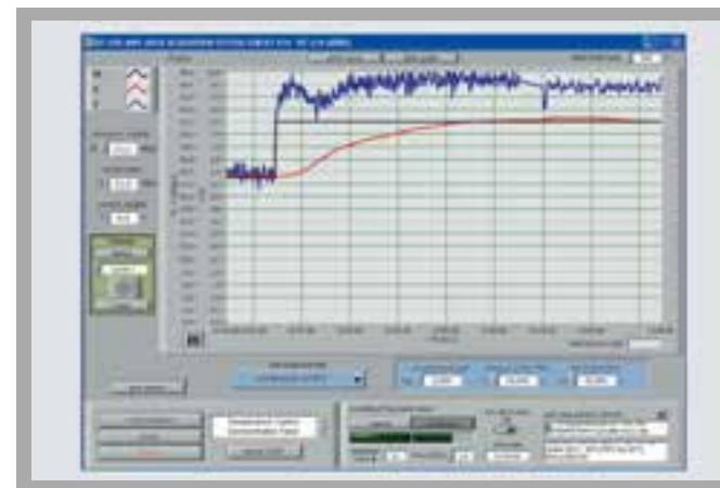
Screenshot of optional I&C software RT 650.40: step response to change in reference variable with PID controller (acceptable control quality)
