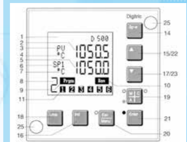
Operation, parameterisation and configuration of a digital industrial controller via keypad
