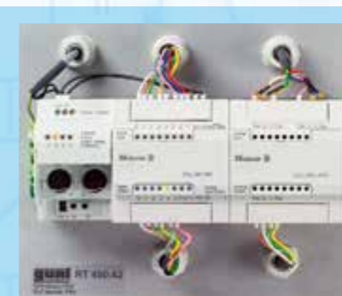
Programmable logic control (PLC)
