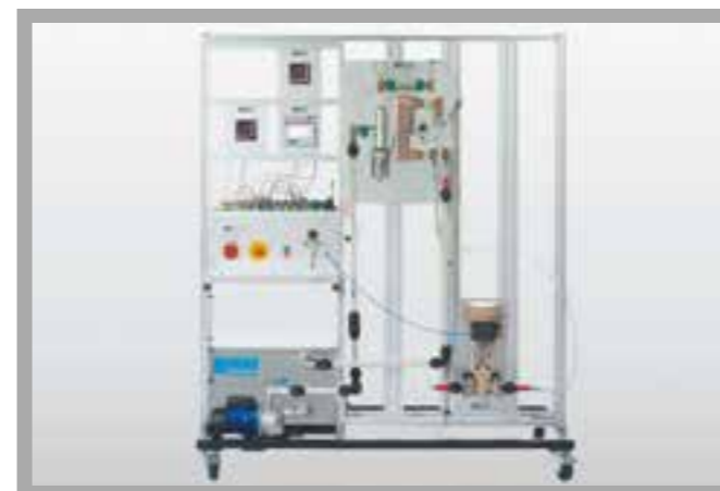
The illustration shows the layout of a temperature control system. In addition to the base module RT 450, it includes the following components: RT 450.04 (controlled system module: temperature), RT 450.11 (controller), RT 450.12 (recorder), RT 450.21 (control valve) and RT 450.36 (temperature sensor).
