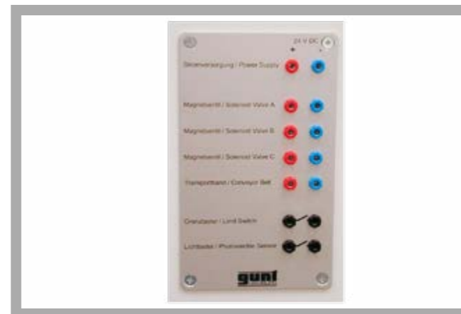
Electrical connections of the solenoid valves and sensors
