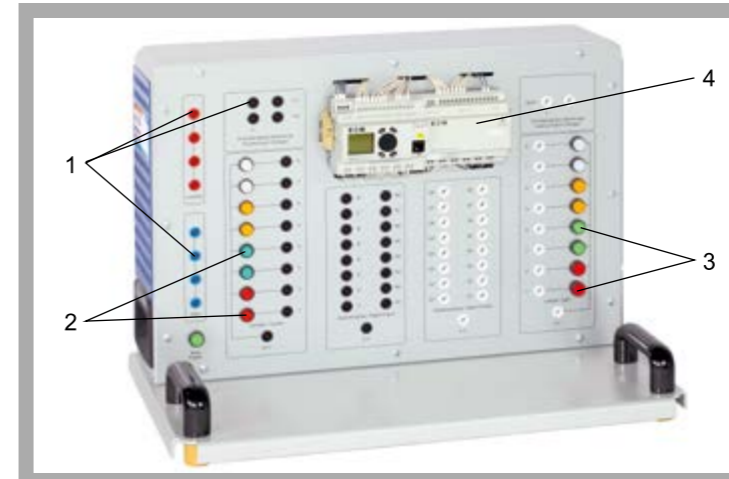
1 lab jacks, 2 pushbutton, 3 lamps, 4 PLC
