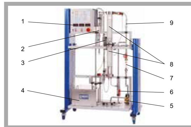
1 digital pressure indicators, 2 air flow meter, 3 compressor for air, 4 storage tank, 5 pump for water, 6 bottom rising-falling switch valve, 7 water flow meter, 8 two-piece packed column, 9 top rising-falling switch valve
