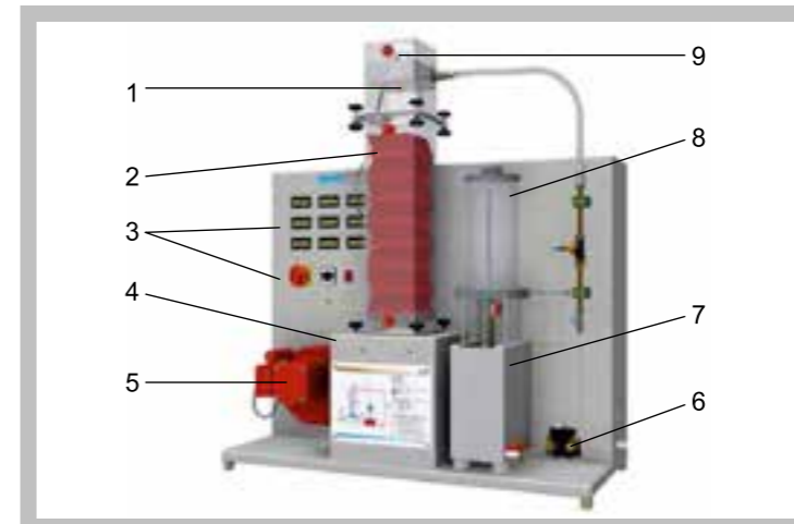
1 nozzle as atomiser, 2 wet deck surface, 3 displays and controls, 4 air chamber, 5 fan with throttle valve, 6 pump, 7 tank with heating, 8 tank for additional water, 9 combined temperature/humidity sensor
