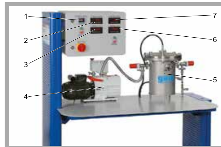
1 temperature controller with temperature display, 2 temperature display, 3 power display, 4 vacuum pump, 5 pressure vessel, 6 vessel's absolute pressure display, 7 vessel's relative pressure display
