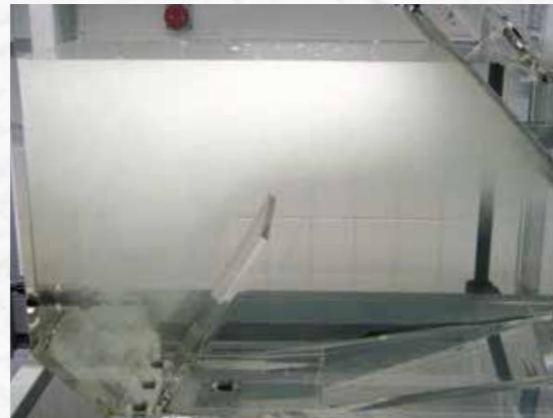
The recycle water enters the flotation tank: The sudden relief to atmospheric pressure causes the dissolved air to precipitate as a cloud of small bubbles.
