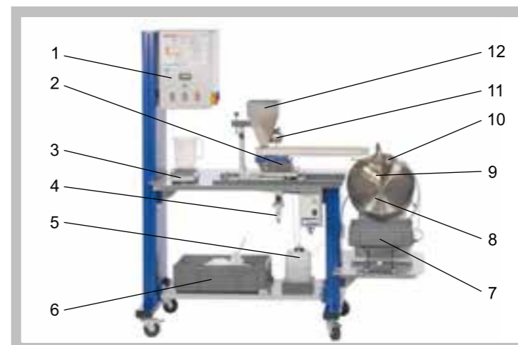
1 switch cabinet, 2 solid material metering device, 3 balance, 4 pressure reducing valve, 5 granulating liquid tank, 6 solids tank, 7 agglomerate tank, 8 dish granulator, 9 scraper, 10 two-component nozzle, 11 vibrator, 12 solids silo
