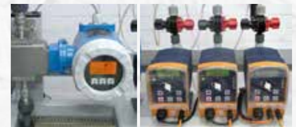
Use of high quality components: Magneto-inductive flow rate sensor and metering pumps
