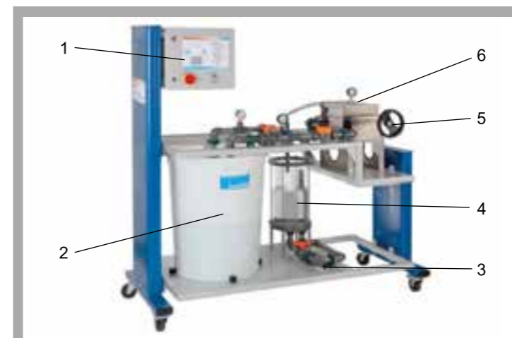
1 switch box with controls, 2 suspension tank, 3 filtrate tank outlet and overflow, 4 filtrate tank, 5 spindle, 6 plate and frame filter press
