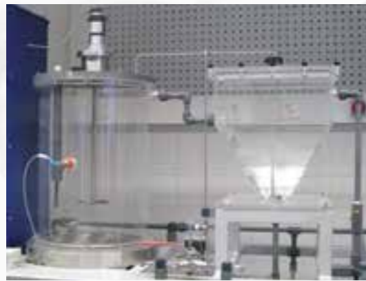
Stirred tank with secondary clarifier
