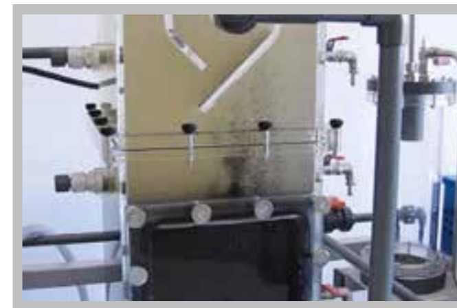
UASB reactor during experimental operation
