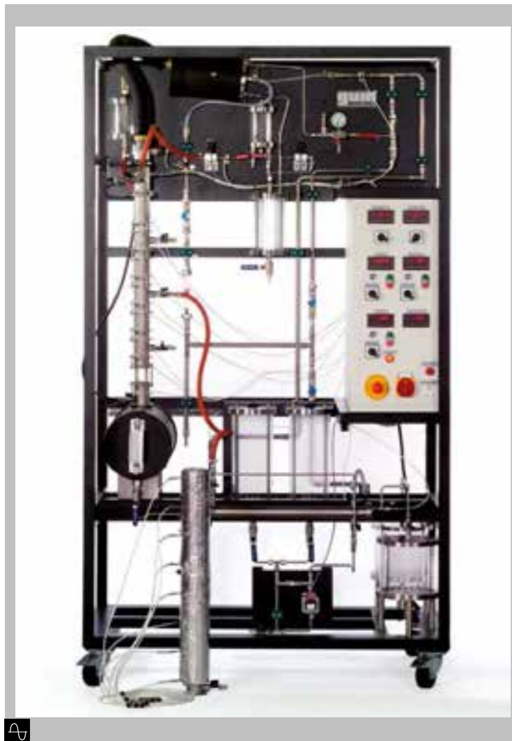
The illustration shows the CE 600 with built in sieve plate column. The packed column can be seen in the foreground.
