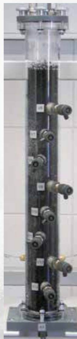
Primary component of CE 583: adsorber with sampling points
