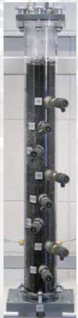
Primary component of CE 583: adsorber with sampling points
