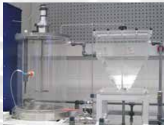
Stirred tank with secondary clarifier
