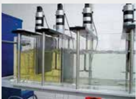
1 Flocculation tank with stirring machines
