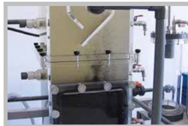
UASB reactor during experimental operation
