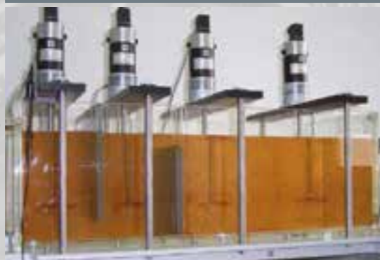
Formation of flocs by coagulation and flocculation
