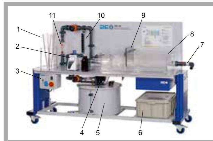
1 suspension flow meter, 2 fresh water flow meter, 3 switch box, 4 bypass valve, 5 suspension pump, 6 suspension tank, 7 storage bin, 8 outlet, 9 sedimentation tank, 10 baffle plate, 11 fresh water/suspension mixing zone
