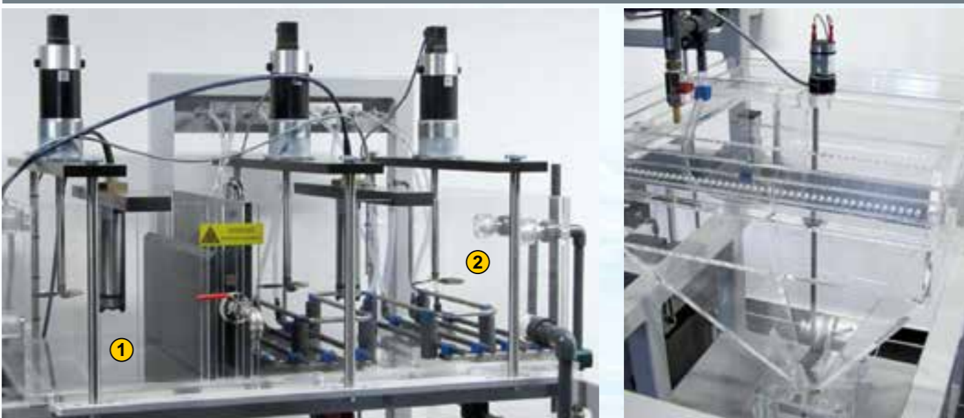
Aeration tank with an aerobic zone (2) and an anoxic zone for pre-denitrification (1)
