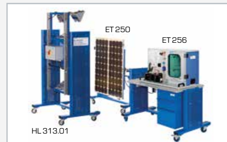
ET 256 together with the optional artificial light source HL 313.01 and solar modules ET 250
