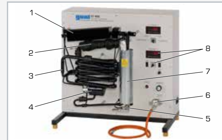
1 condenser, 2 evaporator with heater, 3 absorber, 4 tank, 5 gas burner, 6 pressure reducing valve for propane gas operation, 7 boiler with bubble pump to separate the ammonia, 8 displays and controls
