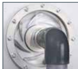
Vanes and impeller of the Francis turbine
