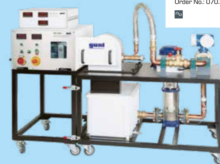
Trainer for turbines with Pelton turbine HM 365.31, supply unit HM 365.32 and brake unit HM 365
