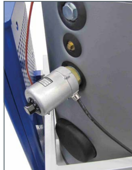
The storage tank is emptied in preparation for the experiment. The auxiliary heater can easily be inserted subsequently in just a few steps.
