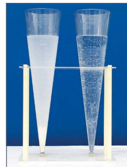
Along with your product, you receive two Imhoff cones to clearly represent and quantify the treatment success of the process.
