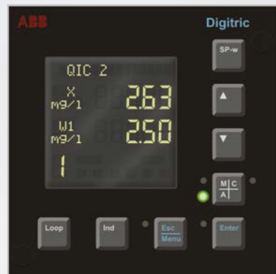
Professional controller for the oxygen concentration in the nitrification area
