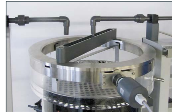
Rotary distributor on the head of the trickling filter with variable speed adjustment
