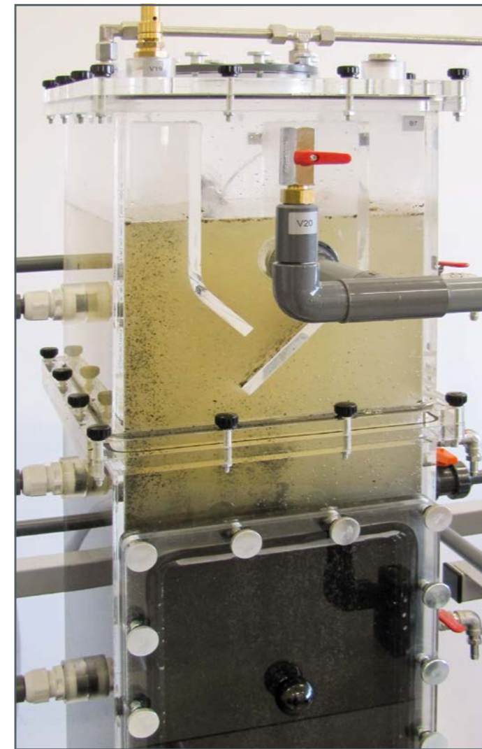
CE702's UASB reactor during a successful trial run in our laboratory
