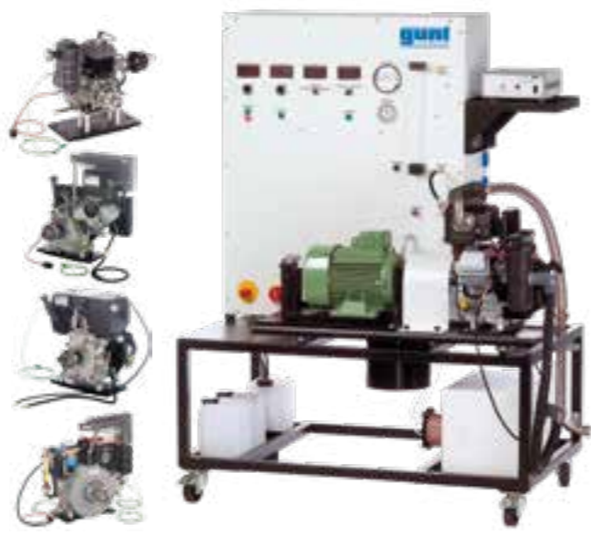
CT 110 Test stand for single-cylinder engines, 7,5kW
