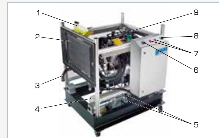
1 cooling water tank, 2 radiator with protective screen, 3 exhaust gas connection, 4 fuel tank, 5 battery with main switch, 6 operating time counter, 7 warning lamps, 8 key switch for ignition, 9 connection for engine feed air
