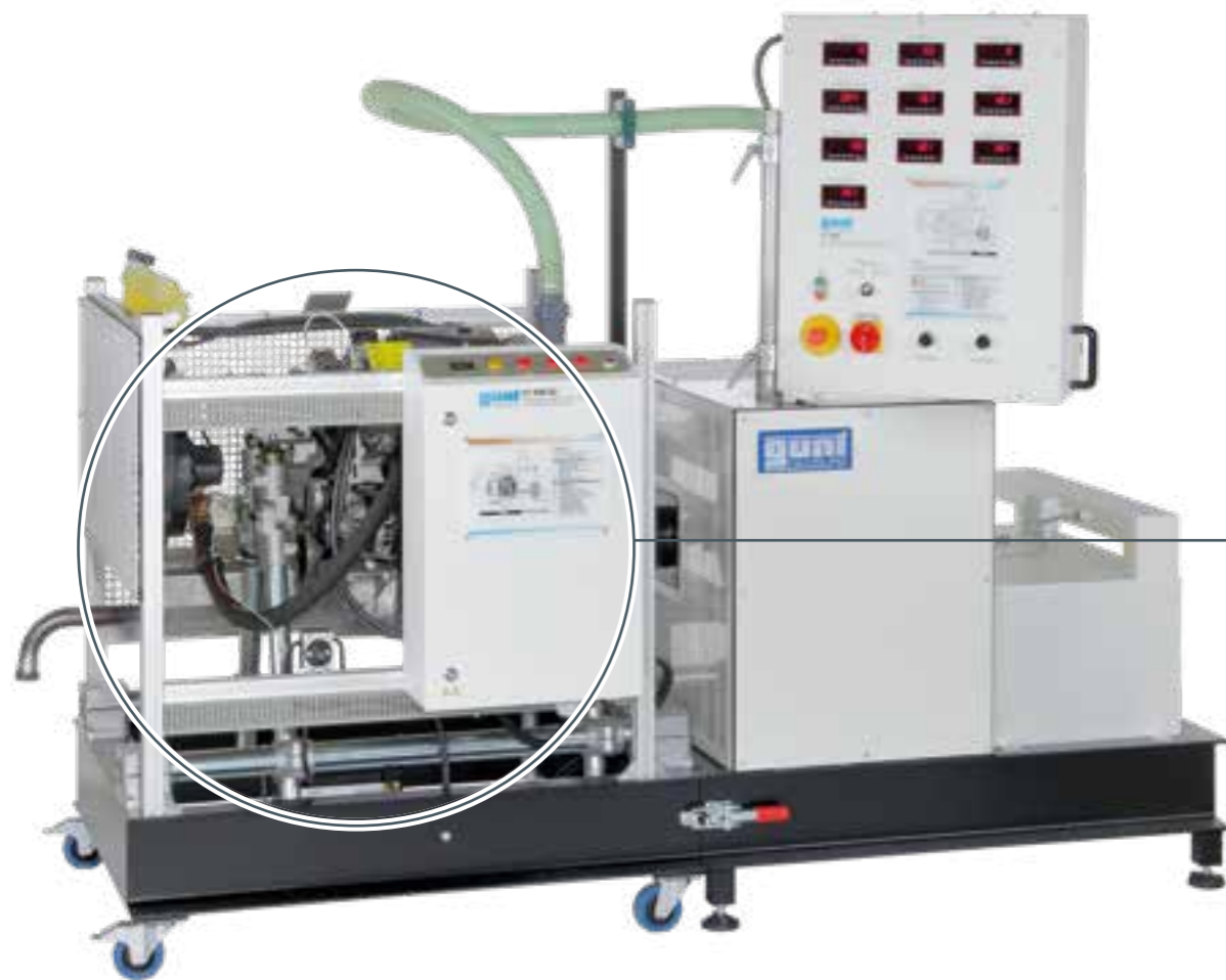
CT 400 Load unit, 75 kW, for four-cylinder engines
