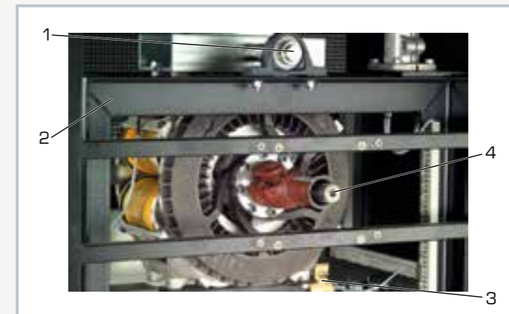
The eddy current brake is mounted in a suspended frame (1 bearing, 2 frame). The supporting force generated by the torque is recorded by a force gauge (3). 4 jointed shaft with spline
