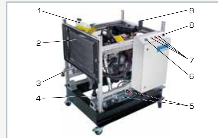
1 cooling water tank, 2 cooler with protective screen, 3 exhaust gas connection, 4 fuel tank, 5 battery with main switch, 6 operating time counter, 7 warning lamps, 8 key switch for ignition, 9 connection for engine feed air
