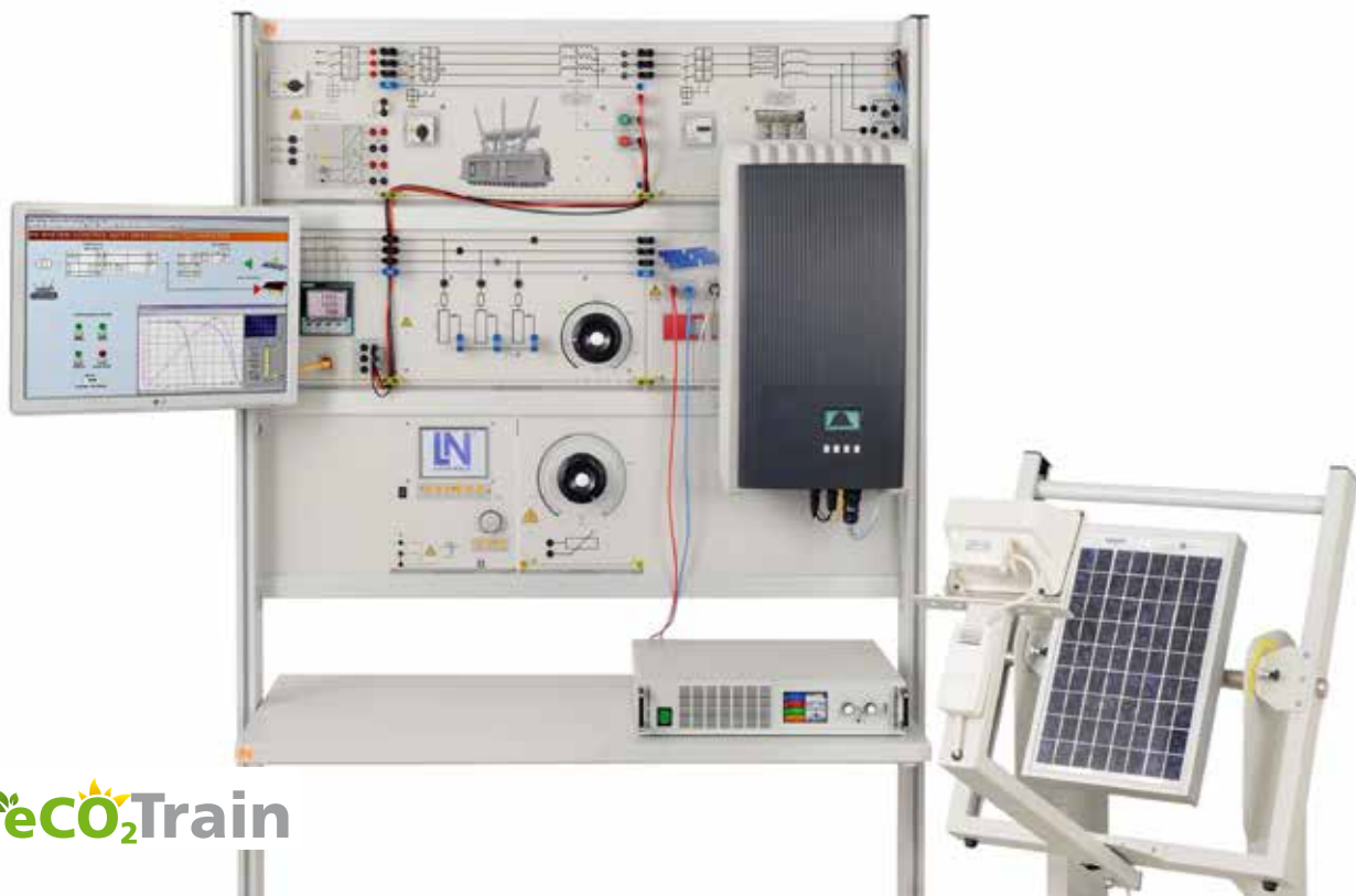
Example experiment: "Setup for photovoltaic systems operating parallel to the grid" EPH 3
