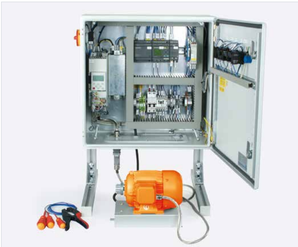
Experiment example: "Project work: industrial wiring of frequency-converter drives EPL 25"
