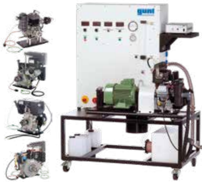
CT 110 Test stand for single-cylinder engines, 7,5kW
