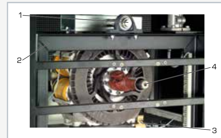
The eddy current brake is mounted in a suspended frame (1 bearing, 2 frame). The supporting force generated by the torque is recorded by a force gauge (3). 4 jointed shaft with spline
