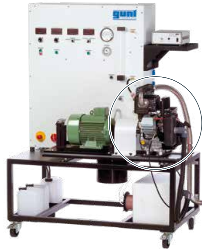
CT 110 Test stand for single-cylinder engines, 7,5kW
