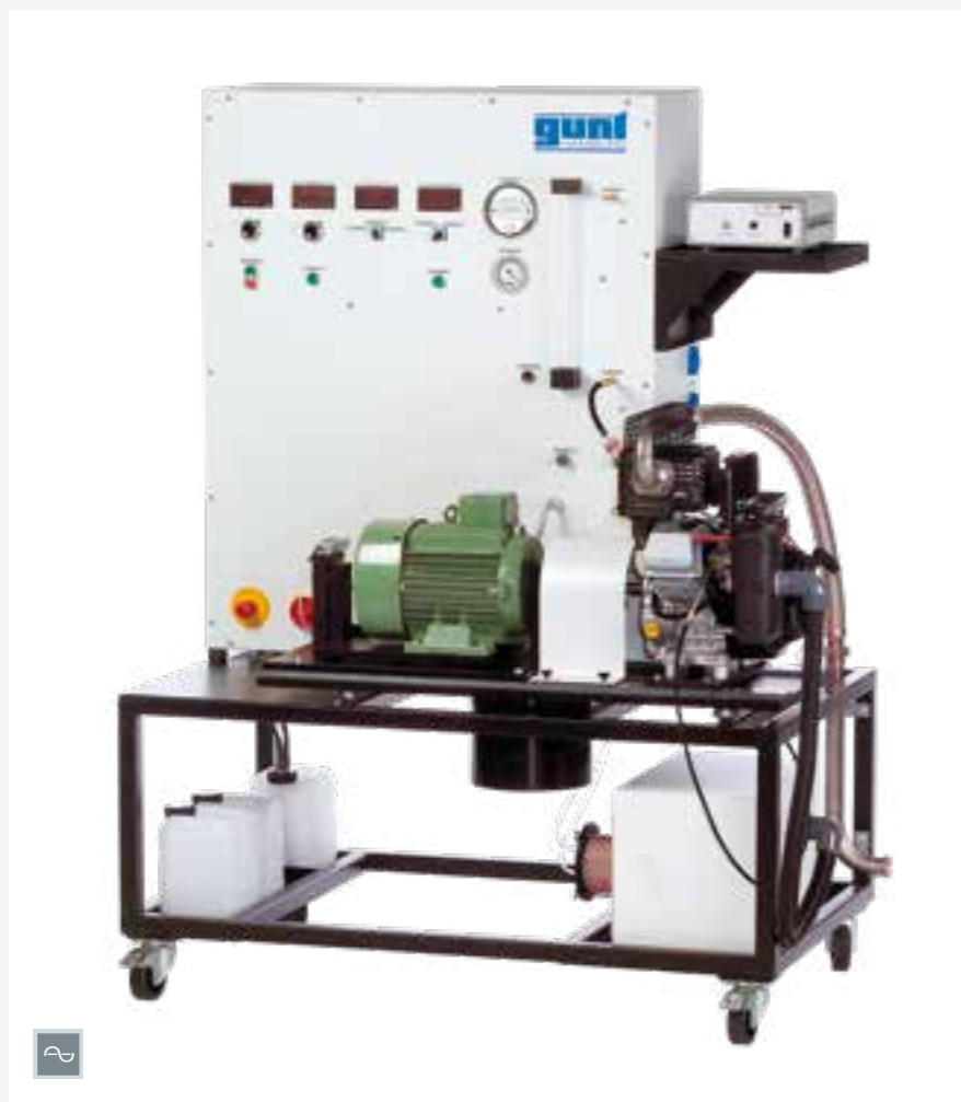
The illustration shows the CT 110 with the CT 100.20 engine and the CT 100.13 electronic indication system (on the shelf).
